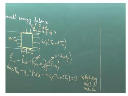
So, let us say that this is the channel and we take a control volume like this. Across this control volume, we are going to write an energy balance, so when we are going to write an energy balance, there is some energy that is entering. Let us say that this length is d x. There is some energy that is leaving, so what is the energy that is entering in terms of the bulk mean temperature.
