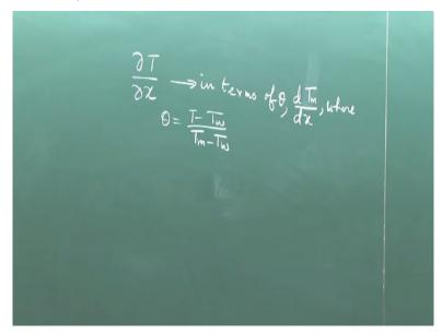
So, for constant wall temperature it is theta into d T m d x and for constant wall heat flux, it is just d T m d x without involving theta that much we discussed in the previous class. Now, irrespective of the boundary condition, this parameter is always involved. So, one thing we have been successful in reducing the dimensionality of the problem that when we are expressing delta T delta x in terms of d T m d x.
