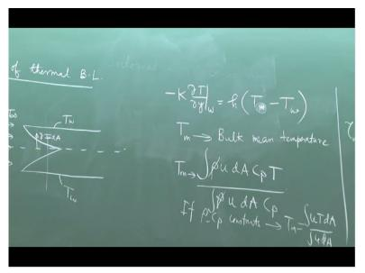
Growth of thermal boundary layer. So, let us say that this fluid which was coming with a velocity u infinity was also coming with a temperature of T infinity and the wall temperature T wall. You may argue that the 2 walls may not be at the same temperature at the undergraduate level, we will not be entering into that complication. We will assume that it is symmetric with respect to the thermal problem also.
