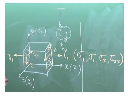
Now, what we will do is we will try to draw the various components of the stress tensor on this element, so let us take this surface. I will just write tau, you have to tell what will be the indices. What will be the first index, first index is normal to the surface, which is under consideration. This surface has normal in what direction? 1, x1 right, so the first index is 1, okay. The second index is what?
