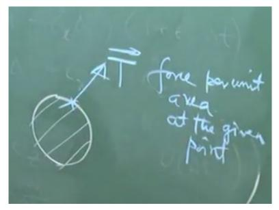
This is a force. This is not actually any external applied force. This force is because of the interaction between the shaded volume with the remaining part of the volume. This is like action reaction type of force, okay. Now, this is not the total force. This force per unit area, okay. So, if this is force per unit area that means the total force will be dependent on the area that is chosen here. Let us say, you choose an area.
