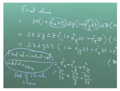
So, this what does it indicate, this is rate of volumetric strain so it is clear from here that this term, which is put in the square bracket represents the rate of volumetric strain. For what kind of situation, you do not have any change in volume of fluid element, when the flow is incompressible.
