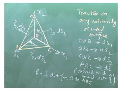
So, to understand that this is the traction on any arbitrary surface, arbitrary oriented surface rather. So, let us that we have a volume taken, which is like this. How many surfaces does this volume have? Four surfaces. Can you tell that why have we chosen this type of surface? So, in this volume, there are three surfaces, which have normals along x1, x2, and x3, but the fourth one is not.
