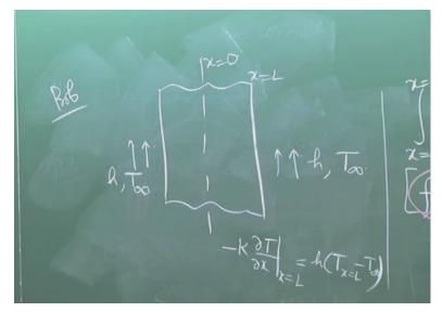
Let us say same infinite slab. Let us say that some fluid is flowing outside the slab with heat transfer coefficient h, and temperature T infinity. So, the only difference from the previous problem is that there is a different boundary condition. Previous problem what type of boundary condition it was? It was a Dirichlet type of boundary condition where the temperature was specified. What type of boundary condition is not there for this problem?
