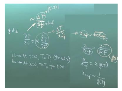
Which property has to be constant for this equation to be satisfied? K, Rho and CP, none of the above, tell? K, right. So, has to be constant. Now, out of other assumption are that the heat conduction in the y and x direction are not important that brings you to the one-dimensional problem. And you have to keep in mind that we are not considering any heat generation in this particular problem.
