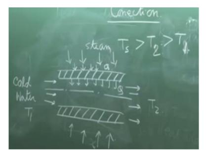
I will give two examples, consider steam condenser in a power plant. You have read power plant in thermodynamics. Let us consider a pipe through which circulating water flows. Let this is the thickness of the pipe, I am showing with little amplification or enlargement for your understanding. This is a pipe typical condenser pipe, there are a number of pipes one pie where the cold water is flowing like this.
