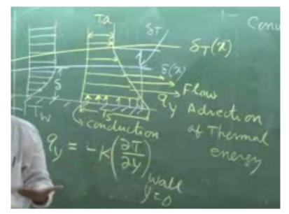
This is the, this value is delta T, this is being reduced while this is reduced mathematically you see the temperature gradient that del T, del Y at the wall is increased. You understand because the thermal boundary layer is reduced that means the fluid attains the cold temperature free stream temperature at a very close distance from the plate, but the plate temperature remains same that means the temperature curve is more steep.
