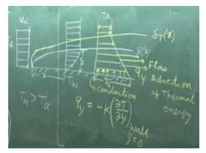
Now which I will explain you now let us consider the plate. Now to understand the mechanism consider the plate at Tw and let us assume that fluid is flowing or approaching to the plate leading edge of the plate with a velocity of U infinity. This is a recapitulation of your basic fluid mechanics concept which you have already read U infinity. And with a uniform temperature of Ta.
