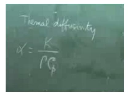
But before I end, I tell you one property known as thermal diffusivity alpha is defined as K/Rho\*Cp where K is the thermal conductivity, Rho is the density and CP is the specific heat at constant pressure. Now you know that there are thermo physical properties of any physical problem related to any physical problem which can be classified into two groups.
