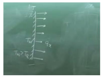
Similar is the case that when you have a vertical plate that I have told earlier at some temperature Tw where Tw is greater than Ta, the heat is transferred by convection in this direction. Here it is qx if we write the heat flux okay. Now the flow situation is like that this is a free convection case and this is a forced convection.
