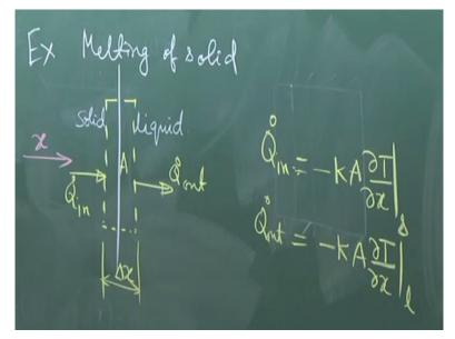
So, we are taking an example which is little bit different this is melting of a solid. So, let us say there is a solid, there is a heat transfer here, let us say it is a 1-dimensional situation. There is a heat transfer along x, so some heat is utilized for melting the solid to liquid. Let us say that we take a small control volume like this surrounding the interface. This control volume is of thickness delta x in the limit as delta x tends to 0 we can recover a sharp interface.
