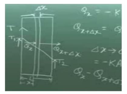
So therefore, for a plane wall with constant thermal conductivity we have a temperature, if you show the temperature scale here this is T1 and this is T2 from any reference datum so we give a linear profile. The slope of which will depend upon the thermal conductivity okay. This is clear, when we have a linear temperature profile. Now in this context, I will tell you certain things okay.
