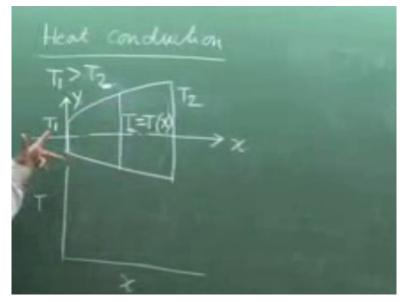
Now if we have a solid like this, whose area is not constant and if we try to conceive one dimensional steady state heat transfer by making this surface that a temperature T1, this is at a temperature T2 so that T1 is greater than T2. Then what will be the temperature variation, will it be linear, will the temperature variation at steady state one dimensional will it be linear no because area is not constant.
