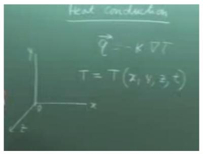
And if we, now think that the heat conduction, heat conduction again then we have seen that the heat flux that is the heat transfer per unit area normal to the direction of heat transfer is minus K gradient of T, where the heat flux is taken as effect. Now therefore, there has to be a temperature variation in this space coordinates. It is a continuous temperature variation for which we can define the gradients that means in the medium.
