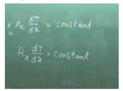
See in this case, I know my basic KAx equation for steady state is dT/dx constant not dT/dx constant. Now if K is constant that we will assume here Ax dT/dx is constant. That means dT/dx is inversely proportional to A. So, such a diverging medium a bar like this, a conical bar so that means temperature variation will be like this. This is T1, (sorry this will go like this) so this is T2.
