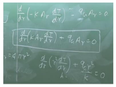
Now Fourier heat conduction equation d/dr of, that is heat flux, heat transfer at any direction is heat flux into the area -qG, Ar is 0, Again and again I am doing the same thing. Now this is not the Fourier heat conduction equation sorry, I am just splitting it heat flux into area, then Fourier heat conduction equation here, heat flux is -K Ar(dT/dr) because heat flux is -K dT/dr.-qG ar is 0, take this – sign out, so that d/dr of K Ar dT/dr + qG\*Ar.
