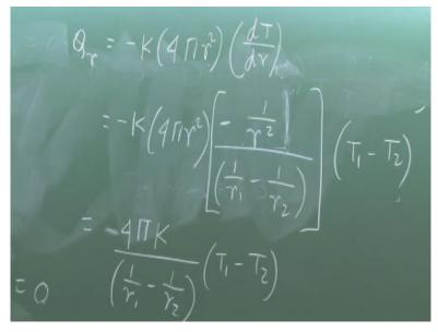
Next part is to find out the heat transfer rate at any radius r, it is =-K\*Area, (4 pi r square) \*dT/dr at r=, sorry not r, at any r, because I am finding out at any current radius which is Ar, 4 pi r square-K(dT/dr), Now what is dT/dr? 4 pi r square, now dT/dr is, there is a – sign, 1/r1-1/r2, so there will be a – sign, so -, dT/dr is 1/r, -1/r, that it 1/r square, - will be there, sorry, that means these r square and r square will cancel out, 4 pi r square.
