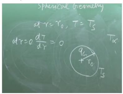
The problem is prescribed that thermal energy is generated at a rate of qG per unit volume which is constant throughout and I have to keep this surface temperature Ts constant, well there is an ambient T infinity which is not very important in determining the temperature distribution, so this is a solid sphere, so the boundary condition requires that at same thing, at r=r0, T=Ts.
