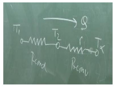
That is r2-r1 as we are generated that is 4 pi K(r1r2) + i/h (4 pi r2 square), this is because heat is, Q is T1-, if I consider this surface temperature is T2, which is not prescribed by, but I can write in these way r2-r1/4 pi K (r1r2) and the same heat is flowing in series under steady state with T2-T infinity1/h, rather it is better to write this fashion, it will be understandable by the definition of h, h\* h\*(2 pi r2 L) \*T2-T infinity T2-T infinity.
