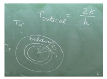
That is all, here also if you add insulating material in the spherical cell, the concept of critical radius of insulation will come and you derive it, it is your task that I will not do, the critical radius of insulation for spherical wall is r critical is 2 K/h, that means if I have a spherical cell or a spherical ball, whatever you call, spherical cell and the problem is prescribe like this, this is r1, the outer radius and heat at a temperature of T1.
