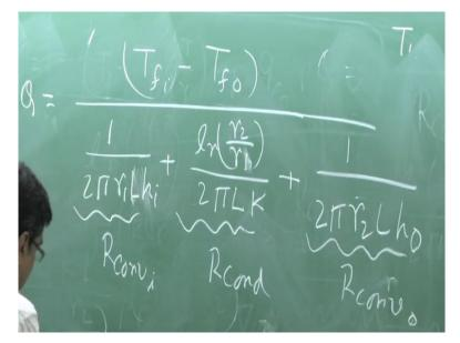
Then we get Q is equal to in terms of the extreme temperature difference, we here prescibe that is Tfi minus Tfo divided by 1 by 2 pi r1 h1 plus ln r2 by r3 divided by twice pi LK, r1 l, sorry twice pi, I am sorry, twice pi r1 L hi plus 1 by twice pi r2 L ho, extremely simple. So, it is the r1 and it is r2, ln r2 by r1, I have written r3, sorry, very good. Now this is same as the flat plane thing.
