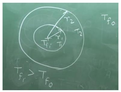
Instead of prescribing the inner surface than outer surface temperature, we prescribe the fluid temperature, inner fluid temperature which may be Tfi and outer fluid temperature which may be Tfo. That means the heat comes from the inner fluid through this, let us consider Tfi fluid temperature inner is greater than Tfo. Then first by convection heat will come to the inner surface and it will have a temperature T1, which is not prescribed.
