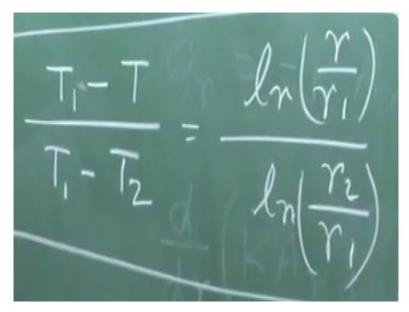
If you use these two boundary conditions, you get a profile temperature distribution T1 minus T divided by T1 minus T2. T1 is the inner surface temperature, which is higher than T2 is equal to ln r by r1 divided by ln r2 by r1. It is very simple that you substitute this to find out T1 and T2. T is equal to T1 ln r1 plus C2 and T2 is T1 ln r2 plus C2 and you can find out T1, T2 and finally you get this as the logarithmic distribution.
