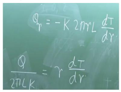
That has any radial location Qr, I know the temperature distribution is written like that, heat flux is K into twice pi r L dT/dx. There is no assumption, Qr is minus K 2 pi r L dT/dx, this is an analog of heat conduction. Now if I neglect heat generation, steady state, we did so many things, but it is a quick approach, that Qr, that is, across any cross section, at any R is constant, that means Qr itself is constant.
