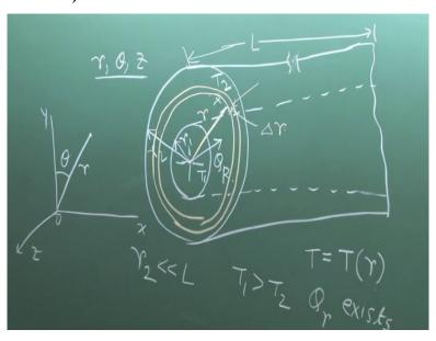
Let us consider a cylinder like this and the problem is specified like this, which we will be discussing. Let this be the center. The cylinder with inside radius r1 is cylindrical tube, outside radius r2, that means this portion is the solid cylindrical wall type of thing and the length of this cylinder is L and the problem is like this, r2 the outside radius of the tube, outer radius is very less than L, that means length is much more than the radius.
