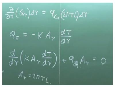
So, if we write this, Qr plus then, we can write del/del r of Qr delta r is equal to qG into twice pi r L delta r. So, this equation is the same as we did for plane wall. Now, we have to replace Qr by food-air conduction equation. What is Qr? At any radius, at an orbit steady location r, Qr is minus K into the cross-sectional area at that r into dT/dr, so therefore if we put that here, now here also twice pi r L, actually it is the cross-sectional area.
