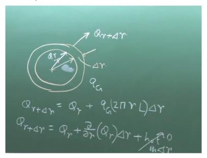
For clarity, I write here the annular ring. This is at an orbit value radius r, with this one delta r, then our same analysis what we do is that if Qr is the heat flux incident on this inner area, then this is the dimension, I am sorry. This Qr is the heat and heat going out is Qr plus delta r. The equation is very simple. If we consider a heat generation per unit volume qG within the cylindrical wall with extent from r1 to r2.
