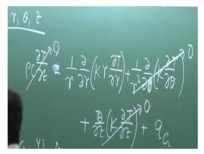
So, in a cylindrical polar coordinate system, r theta z. If we write this divergent K grad T, then it will be like this, rho C del T/del t is equal to 1 by r, I think you know this thing, del/del r of Kr del T/del r plus 1 by r square del/del theta of K del T/del theta plus del/del z of K del T/del z plus qG. That means, in a cylindrical polar coordinate system, if we define a cylindrical polar coordinate system like this, in x-y plane.
