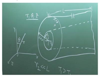
This can be expressed in terms of cylindrical coordinate system if it is sufficient coordinate the r, this is the polar azimuthal angle theta and z, r, theta and z. The coordinate system, in which any point here in the cylindrical wall, r1 to r2 can be specified, where z is the coordinate along the length and r and theta the radial and azimuthal coordinate.
