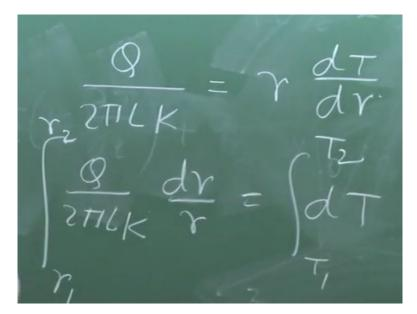
Now if I integrate this from r1 to r2, inner to outer, and a variability T1 to T2, and with this consideration, that Q is constant, which is not varying in the radial direction, because for a steady state heat transfer without heat generation same heat has to pass through each and every perception. In the similar way, I told for plane wall also it can be done like that, in many books it is done like that.
