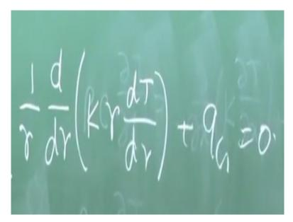
That means this equation becomes 1 by r and del/del r, you write d/dr, that means from the general heat conduction equation we can also get the same expression that is 1 by r d/dr of Kr dT/dr plus qG is 0, so this is my one-dimensional steady heat conduction in a cylindrical wall. It is as simple as that. Another way of deriving this equation is the same. This is the most simple and intelligent way.
