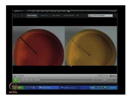
So, let us look into one example or rather 2 examples shown side by side, these are 2 fluids with 2 different viscosities there is a line colored line which is moving with the shear and that is a line which sort of represents the deformation and we just see it again hopefully it works. Now, can you tell from these 2 examples just qualitatively whether the red one has more viscosity or the yellow one has more viscosity?
