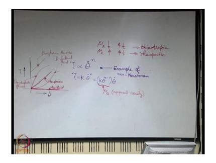
One of the examples is like you may have the shear stress is related to a power of the rate of deformation that is  $\tau \alpha \dot{\theta}^n$ .
