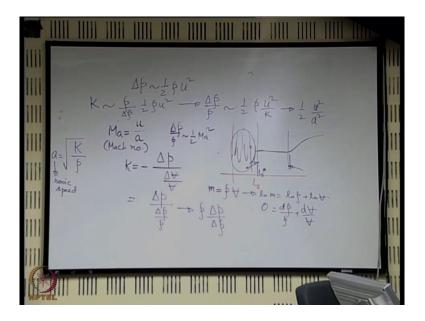
So, in the numerator you have u in the denominator you have a. So, u is the velocity of flow and a is the velocity of a disturbance, which is moving in the medium in which the flow is occurring and these 2 ratios is known as Mach number.
