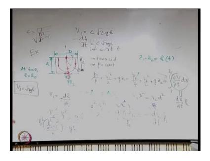
Let us say that now this height is h which is changing with time. So, there is no hole here but there is some hole here. There is a nozzle that is fitted and water is coming out, ok. So, when you are doing that the way in which most of you have done is like you have assumed the velocity  $V_2 = \sqrt{2gh}$  this is known as Torricelli's formula.
