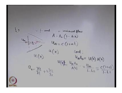
And it is carrying a fluid with density equal to constant and some other input data are given for the problem. The area of the cross section of the nozzle, it varies with the area of the cross section of the inlet by  $A = A_0(1-bx)$ ,  $u_{\infty} = c(1+at)$ . What we are asked to find out that what is the acceleration as a function of x.
