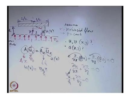
Now, say the top plate is a rectangular plate with the dotted line representing the axis of symmetry. The bottom plate is a very special plate. It has some holes; we call it a porous plate. So, it has some pores or holes and the idea of keeping these holes is to blow some fluid. We will see that it is not just a mathematical, mathematically defined idealistic problem. Many times, it is something which is followed in technology.
