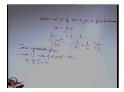
So, incompressible flow, it will have what signature? One and only important signature 0 rate of volumetric strain because the fluid element may not be changing its volume that is the meaning of that is even the literal meaning of incompressible that you cannot really compress it.
