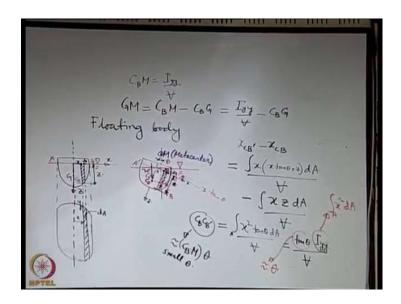
So, if you recall this sketch which we were discussing in the previous class, we identified a point known as metacenter and the motivation behind identifying this point is that when it's a floating body and it gets displaced and its submerged portion within the water changes its configuration. The centre of buoyancy does not remain fixed at its own position. So, referring to a fixed centre of buoyancy, might not work as a stability criterion.
