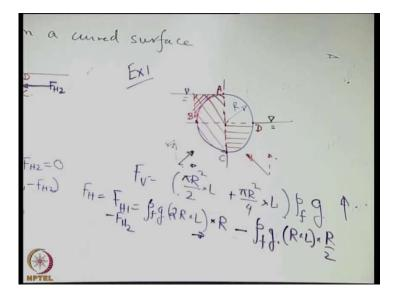
Let us say that we have a long circular cylinder and you have the free surface of the fluid in this way. So, on the left side the this is the free surface on the right side this is the free surface and solid material is a circular cylinder its length is perpendicular to the plain of the board. We are interested to find out what is the resultant horizontal and vertical component of force exerted by the fluid on this cylinder.
