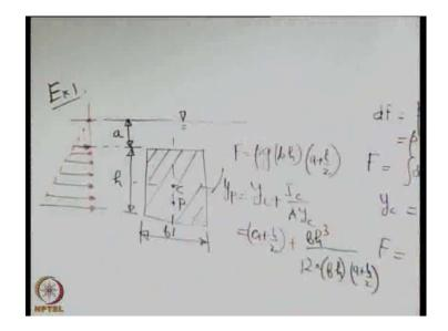
Let us say that you have a surface which in its sectional view is like this. And this is the vertical surface immersed in a fluid. So, this is the fluid. And this subject is a or like this object is a rectangular section with the dimensions b and h. What is the resultant force due to pressure acting on this, let us give a dimension of this say a, this is example 1. The question is, what is the resultant force on this shaded surface because of pressure.
