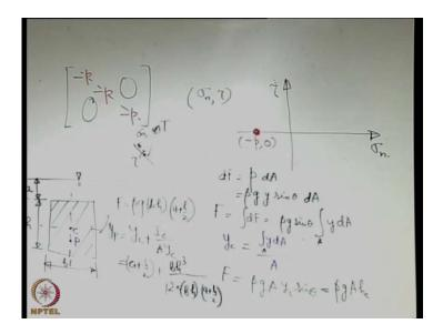
So, we are having two axis, one is  $\sigma_n$  and another is  $\tau$ . Our locus is or our objective is to find the locus of  $\sigma_n$  versus  $\tau$  or  $\tau$  versus  $\sigma_n$ . So, how will the Mohr circle look like for such a state of stress this state of stress is a very unique one. And this is known as hydrostatic state of stress the reason is obvious it represents a hydrostatic physical situation.
