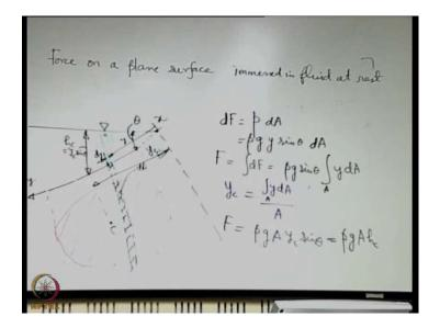
We start with an example of force on a plane surface. What is the special characteristic of the plane surface that is such a surface that we are considering that is immersed in fluid at rest. We will try to make a sketch of the arrangement. Let us say that this is the free surface of the fluid that means on the top there may be atmosphere, in the bottom there may be water as an example. There is a surface the edge view of the surface is like this it is a plane surface.
