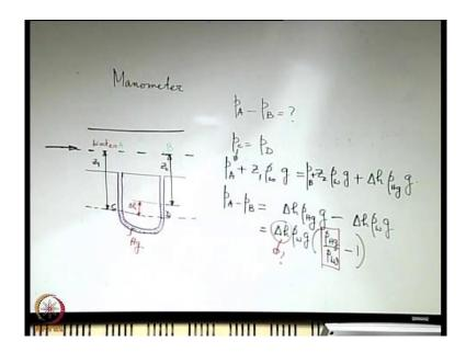
In the last class we say the example of a barometer; today we will first see the example of a manometer. Since this concept is well known to you we will briefly recapitulate it through an example. Let us say that there is a pipe and there is some fluid which is entering the pipe there are two different sections say marked by A and B and we are interested to find out what is the difference in pressure across these two. To do that what we will do?
