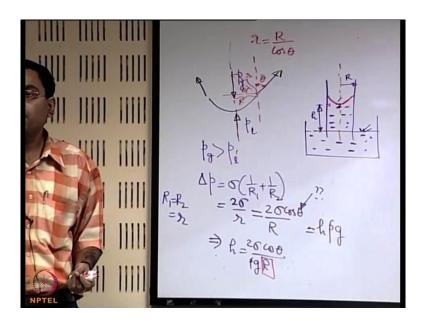
To do that we will take an example when there is a capillary tube which is small in radius. It is dipped into larger volume of fluid, and let us say that this was the initial level of the fluid. And now once this capillary is introduced this fluid is expected to either rise or fall and we will see that what dictates that it should rise or fall.
