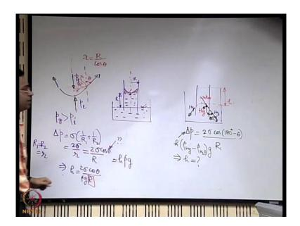
So, let us say that you have a capillary tube, in the capillary tube now you have two liquids on the top you have water and in the bottom you have mercury; with a given tube materials say it is glass it assumes this particular meniscus shape. The outside is filled up with mercury, so there is mercury in the outside and water is being poured from inside.
