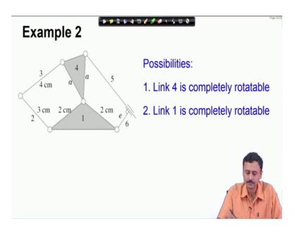
The first case that I am considering is link 4 is completely rotatable which means that a is the shortest link so, this is one possibility the other possibility is link 1 is completely rotatable. So, which means this 2 centimeter link is the shortest link.
