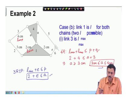
The first case is link 3 is 1 max therefore, this is 1 min and this is 1 max the 4 centimeter long link is 1 max. So, from the 4 R chain side 1 min plus 1 max should be less than equal to p plus q. So, 1 min is 2 centimeter plus 1 max is 4 centimeter should be less than equal to a plus 3. This implies a should be greater than equal to 3 centimeter, but definitely a cannot exceed 4 centimeters therefore, the complete range for a is this so, a must lie between 3 centimeter 4 centimeter.
