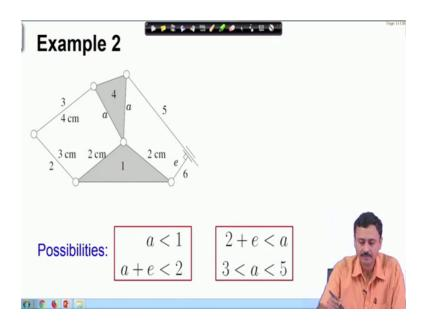
Now, we need to combine you recall that in case a we had this condition. So, here 0 is less than equal to this is so, a must lie between 0 and 1 centimeter and a plus e should be less than equal to 2 and in case b we had 2 plus e should be less than equal to a and a must lie between 3 and 5 centimeter, you can easily draw these regions. So, I have drawn these regions out for you.
