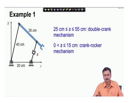
So, here I have recapitulated in the results. So, when s is lies between 25 centimeter and 55 centimeter, we have a double crank mechanism and if s lies between 0 and 15 centimeter then it is a crank rocker mechanism.
