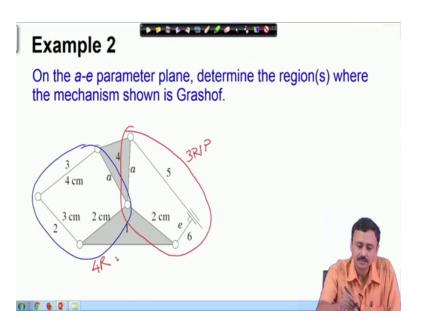
Let us move to this next example here, I have a mechanism that involves the 4 r. So, this is a 4 R chain coupled with a 3 R 1 P chain. So, we have a coupled 4 R and 3 R 1 P chains in this example the problem says on the a e parameter plane.
