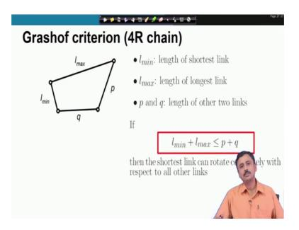
We had discussed about the Grashof criterion for a 4R kinematic chain and this is shown here, if the sum of the length of the minimum or the shortest link plus the length of the longest link is less than the sum of the other two links then the shortest link is a crank.
