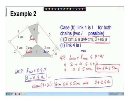
Now, suppose I consider the case that link 4 is 1 max. Therefore, this is 1 min and this is 1 max, if this is 1 max then a must definitely be greater than 4 centimeter. So, from the 4 R chain side 1 min is 2 plus 1 max is a should be less than or equal to 7 that gives us a should be less than a or equal to 5 centimeter. Now, here a is 1 max so, therefore, it has to be greater than 4 centimeter. So, that complete range for a is given by this; so, a must lie between 4 centimeter and 5 centimeter.
