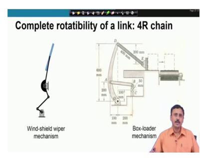
Why or in works what kind of applications do we require this complete rotatibility, here I have shown two examples the windshield wiper which is driven by a motor, it is continuously rotating and the wiper is oscillating. The other was the box loader
