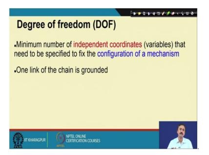
So, what is degree of freedom? The definition is the minimum number of independent coordinates, or variables that need to be specified to fix the configuration of a mechanism, here there are some key words.
