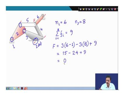
Now, this is another kinematic chain, let us number the links ground is 1 2 3 4 5 6 in this chain therefore, there are 6 links n L equal to 6 number of kinematic pairs, here there is 1 revolute 2 3, this is the contact between link 3 and the ground so, there is a third kinematic pair 4.
