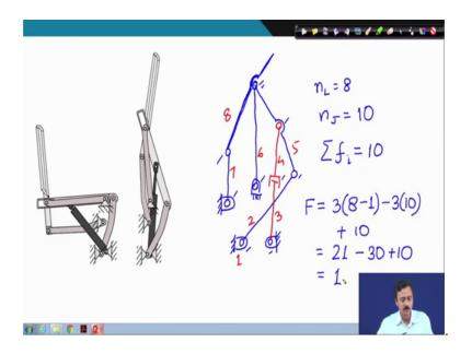
This is the transfer aid there are 4 ground hinges, here we have 1 link, this is the actuator, this is the backrest this is a single link.
