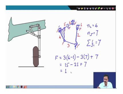
This is the landing gear of the aircraft, there are 3 ground hinges, the ternary link connected to the actuator and this is the wheel.
