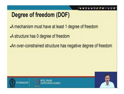
Now, when do we call a chain a mechanism? So, the criterion for naming a chain as a mechanism, is when it has at least 1 degree of freedom. So, it must have at least 1 degree of freedom, then we call it a mechanism.
