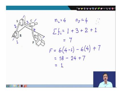
Let us discuss some examples of spatial kinematic chains, let me count the links ground is 1 2 3 and 4. So, number of links is 4 number of joints we have a revolute here a spheric 2, a cylindric 3 and a prismatic 4. So, number of joints is 4 and summation of degree of freedom of all joints, let me do this calculation here.
