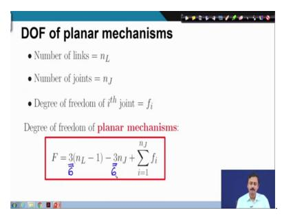
So, this is the formal way we have derived the degree of freedom calculation. So, if the number of links is n L number of joints is n J. And the degree of freedom of the ith joint is f i, then the degree of freedom of a planar mechanism is 3 times n L minus 1 minus 3 times n J plus summation of degree of freedom of individual kinematic pair.
