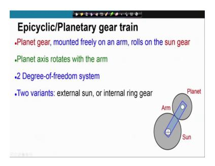
Then, epicyclic gear train as I have mentioned that there are gears who centres can move or rotate in space. This is unlike the simple and the compound gear trains where their centres are fixed. The epicyclic gear train has these components, it has got planet gear which is mounted freely on an arm and it rolls on what is known as the sun gear. This is the analogy is from our solar system.
