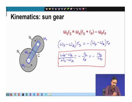
If you do that, then omega S r S must be equal to omega A r S plus r P minus omega P r P. Now, if you simplify this expression, you can write this as omega S omega S minus omega A times r S is equal to minus of omega P minus omega A r P. So, therefore, now I can take the ratio let us say omega P minus omega A by omega S minus omega A that is equal to minus of r S by r P and this you also know is equal to minus of N S by N P.
