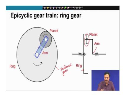
This is the second type in which we have a ring here. So, this is an epicyclic gear train with a ring gear this is an internal gear, so, the ring gear is an internal gear. If you look at the schematic representation, this is the ring gear and we have the planet mounted freely on the arm.
