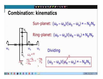
So, omega all the gears move at the same angular speed omega R is equal to omega A is equal to omega S. If I let us I fix the ring gear; let us say if I fix the ring gear which means I do not allow this to rotate, then I have this relation omega sun minus omega arm by minus omega a is minus N R by N S. So, now various combinations you can calculate the relation between the gears the angular speeds of the gears.
