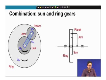
Let us now look at the combination of both sun gear and a ring gear with a planet. Now this is the fundamental unit that is used in automatic transmission as we will discuss. This is the schematic representation of the gear train with this combination of ring and the sun.
