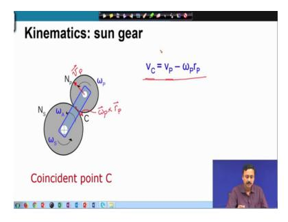
Let us now look at the kinematics of the epicyclic gear train. In order to derive the relation between the input and out now, we know that there are 2 inputs and 1 output just 2 degrees-of-freedom. Therefore, we consider this contact point C of the pitch circles of the sun and the planet gears and trying to do a velocity matching at the contact; this is for pure rolling.
