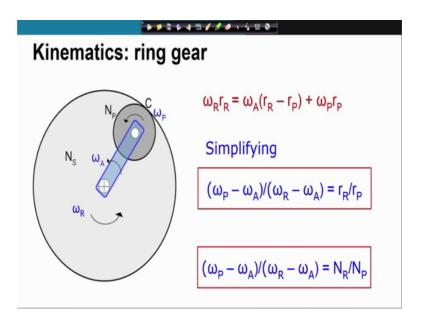
If you simplify this expression, we have this relation and you can write this ratio of the on the right hand side r R by r P as N R by N P. Here you should notice that because this ring gear being internal gear, the sign here is positive. This is unlike the relation we obtained when we had a sun gear. So, that completes the kinematics of the epicyclic gear train.
