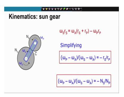
So, this I write out for you. So, this is the final expression of the motion relation. From here given let us say omega of the arm and omega of the sun, you can find out omega of the planet or given the omega of the planet and omega of the sun, you can find out omega of the arm.
