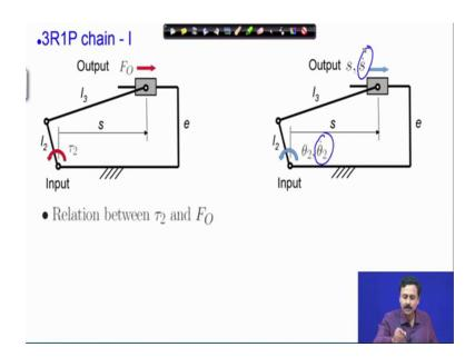
So, here I have shown you 3 R 1 P chain of type 1 and as you can see I have marked the input and the output. So, at the input I have a torque tau 2 and at the output I have a force F O. The force and the output and we have to find the relation between tau 2 and F O. Now, from the kinematics from the velocity relations we had already related theta 2 dot
