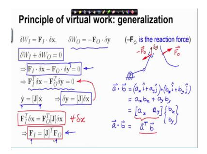
So, in order to generalize our force analysis I have written out the virtual work done at the input delta W I is F I dot delta x. So, delta x is the virtual displacement at the inputs and F I is the force vector at the input. At the output we have F naught as the force being applied. So, if I consider for example, a manipulator the 2 are manipulator let us say, which we are going to look at very soon.
