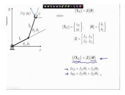
Now, starting from there we can now write the virtual displacement relations when we freeze time and provide an arbitrary input virtual displacement delta theta. And, obtain the corresponding output virtual displacement delta X E. And, they are related through the Jacobian as we observed here. So, the implication is like this that delta x E is J 1 1
