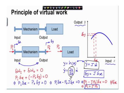
So, let us look at this once again through a schematic figure as I have shown here. Here, I have a mechanism and imagine mechanism shown as a block which has an input and a output at the input let us say we have applied a force P i, which is being transformed and transmitted to the load as P o, which is doing certain work on the load. Therefore, the mechanism feels a negative force P o so, P o in the opposite direction. So, that is the reaction force on the mechanism.
