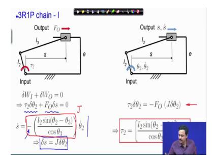
So, then if we proceed further the statement of principle of virtual work says that delta W I plus delta W I equal to 0 where delta W I is the virtual work at the input a virtual work at the input, you can say is tau 2 times delta theta 2. And, virtual work at the output is F O times delta S, you can very easily come to this statement by noticing that tau 2 and theta 2 dot, they are the same direction and F o and S dot have been considered in a same direction.
