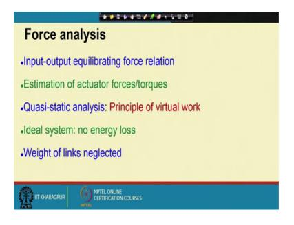
We have discuss that, the input output equilibrating forces is what we are interested in this helps in us in estimating the actuator forces or torques required. We will use the quasi static analysis using the principle of virtual work; that means, there is no dynamic forces in our analysis. We will consider ideal systems, which means that there is no energy loss, there is no dissipation. The weight of the links are neglected in this analysis.
