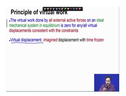
Now, let us review the principle of virtual work, the statement of the principle of virtual work states, that the virtual work done by all external active forces on an ideal mechanical system in equilibrium is 0, for any or all virtual displacements consistent with the constraints. So, here a very important term is this virtual displacement.
