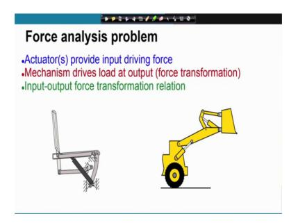
So, let us recapitulate what we have discussed, the force analysis problems, the problem is about finding the input output force relation for a mechanism. In a mechanism or in a robot the actuators provide the input driving force and the mechanism drives certain load at the output. So, the mechanism is responsible for the force transmission and transformation. So, the objective of force analysis is to find this input output force relation.
