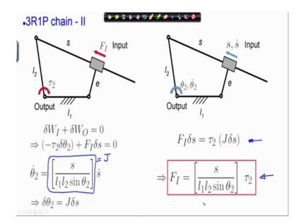
And from here follows the virtual displacement relations delta theta 2 is Jacobian times delta S, now here we have the Jacobian. So, therefore, from the statement of virtual work by replacing this delta theta 2 I have obtained this relation.
