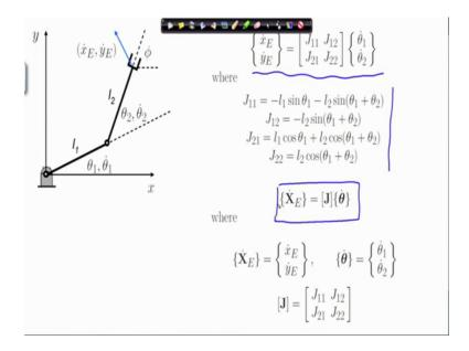
So, we know that the velocity vector at the output is related to the joint velocities at the input through this Jacobian relation, where the Jacobian elements are given here. So, this we wrote in a compact form as X E vector dot is J times theta dot.
