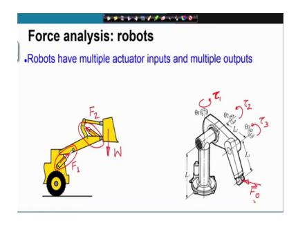
Now, we will look at the force analysis for robots, as you know robots have multiple actuators as inputs and there can be multiple outputs. For example, here we have this excavator we have a load maybe W and we have 2 actuators, which are applying forces F 1 and F 2 and that is responsible for equilibrating the load W.
