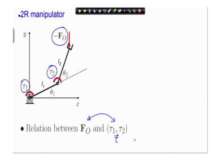
So, here I have a schematic for the 2 R manipulator we have these input forces which are the joint torques tau 1 and tau 2. And, the reaction force that is experienced by the manipulate the at the end effecter which is minus F O, I have to find the relation between this F O and therefore, vector and the joint torque vector tau. Now, we go through the velocity analysis that we have already discussed.
