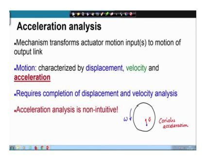
And, that is of a disc that is rotating at a constant speed and a particle that is moving with respect to the disc also at a constant speed. Let us say so even though speeds here are all constant, the angular speed is constant, the linear speed of the particle with respect to the disc is constant, the particle still suffers acceleration and this is the coriolis acceleration as you know. So, the particles suffer coriolis acceleration. So therefore, the acceleration analysis is non-intuitive.
