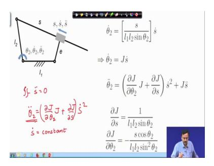
Similarly, if I have the input as a constant which means if s double dot is 0, that means the prismatic actuator is expanding at a constant rate in that case I have acceleration at the output. If I am moving at a constant if I have the prismatic actuator expand at a constant rate which means s dot is constant then the output has an angular acceleration.
