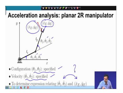
Next let us look at the acceleration analysis of a planar 2 R manipulator. So, here I have shown a 2 R manipulator which is moving at a certain configuration it is moving with velocity theta 1 dot theta 2 dot and acceleration theta 1 double dot and theta 2 double dot.
