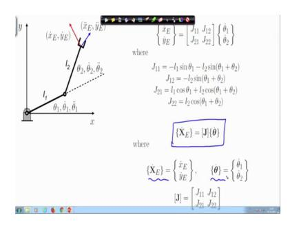
This can be written in a compact form as shown here where  $x \in dot$  this is the endeffector velocity vector and this theta dot vector is the joint velocity vector.
