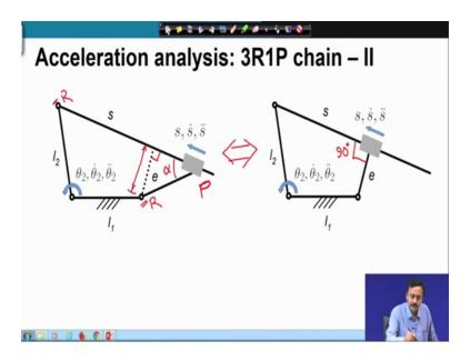
We will start with the acceleration analysis of a 3R1P chain of type 2; we have discussed this point before that for a 3R1P chain of type 2 here we have the offset. So, this is the distance between the 2 revolute pairs connected to the ends of the links with the prismatic pair. So, here we have the prismatic pair and these are the 2 revolute pairs
