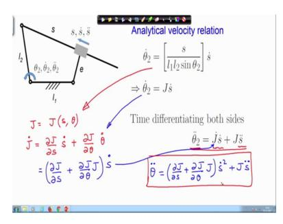
So, if you differentiate with respect to time both sides of this velocity relation you will obtain this acceleration relation. So, on the left I have the acceleration at the output and on the right I have a term where I have the time derivative for the Jacobian and the rate of expansion of the actuator and a term which involves the acceleration of expansion of the actuator.
