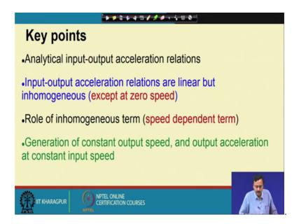
So, what are the key points that we have found we have derived the analytical input output acceleration relations. We are found that the input output acceleration relations are linear though they are inhomogeneous, except at 0 input speed, thirdly we have looked at
