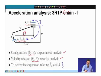
Now, let us go over to the acceleration analysis of 3R1P chain of type 1. So, here we already have completed the displacement analysis, so which I which means I know the input output displacements, I have completed the velocity analysis which means I can relate theta 2 dot and S dot the output is S and the rates are S, S dot and S double dot the input is theta 2 and the input rates are theta 2 dot and the acceleration is theta 2 double
