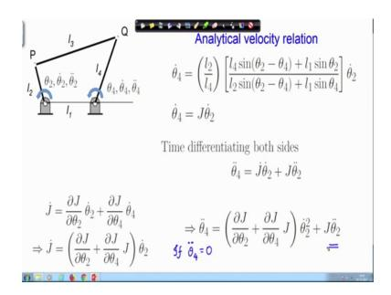
If I need, if I need the output acceleration to be 0 then I require an input acceleration, so what acceleration do I need so let us do this.
