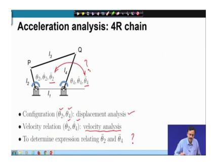
So, here I have an image of this 4R chain. We already know the configuration. So, theta 2 and theta 4 are given and this relation is through the displacement analysis from the velocity analysis we know the relation between theta 2 dot and theta 4 dot. Then we have to find out the relation between theta 2 double dot and theta 4 double dot, so we have to relate these 2. So, this is our Acceleration analysis problem.
