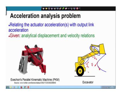
So, what we need is to understand the acceleration input output relation. So, the acceleration problem analysis problem is essentially relating the actuator acceleration with output link acceleration, so this is what the problem is about. So, what are they
