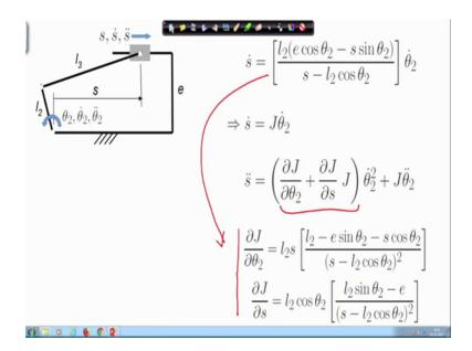
So, here I have written out for you the expressions of del J del theta 2 and del J del S which is required in this term of acceleration relation. So, this can be obtained directly from here by taking this partial derivatives.
