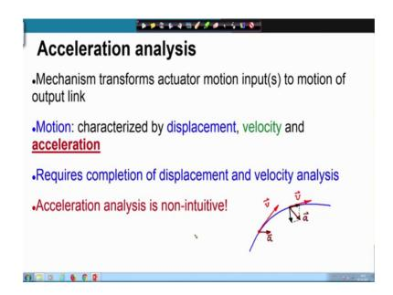
Now, as you know that a mechanism transforms actuator motion which are the inputs to motion of the output link. Now motion is characterized by displacement, velocity and acceleration. So, we have discussed displacement, we have discussed velocity, so these 2 characterize motion. The next characterization comes from acceleration. So, in acceleration we assume that the displacement and velocity analysis has been completed.
