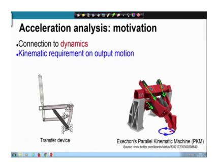
The same holds for this parallel kinematic machine, suppose I want to move the tool on a certain circular path, let us at a constant speed even though the tooltip is moving at a constant speed on a circular path it has acceleration the centripetal acceleration. So therefore, I must have certain acceleration at the actuator expansion as well.
