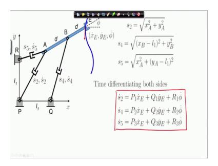
Then I obtain the velocity relations between the end-effector velocity vector and the actuator expansion rates.
