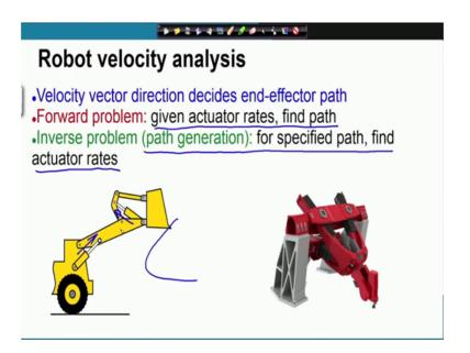
So, as I have mentioned that the velocity analysis problem in the case of robots is also closely related to the path generation problem, so given the actuator rates or the rates at which the actuators are expanding or rotating, we can find the path that the end-effector takes.
