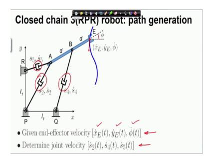
Now, let us look at the close chain 3 RPR manipulator, here this manipulator has 3 degrees of freedom, we are specified the velocity of the end-effector point, the velocity trajectory of the end-effector point though x E dot y E dot and phi dot.
