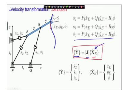
So, here we are defined the Jacobian which relates the actuator expansion rate and the end-effector velocity vector. Here this is quite straight forward because we will have the end-effector velocity vector already specified through the path. So, this vector on the right X E dot will be specified this is known to us, given the path we can find this vector once we plan the time of motion. Therefore, we can directly find out the expansion rates
