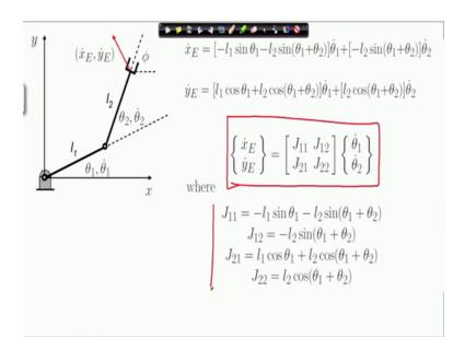
Then differentiating the displacement relations we arrived at the velocity relation, input output velocity relation. So, on the left I have the end-effector velocity vector and on the right I have relation through the Jacobian to the joint velocity vector. Whether an element of the Jacobian for the 2R manipulator has been written out, this we have discussed already.
