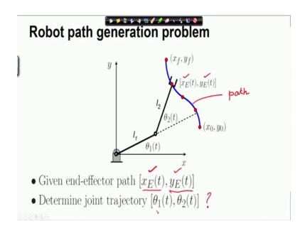
So, this is the problem of path generation, so essentially this is the second and third path. So, what we have is we have the path already specified or determined. Now we have to specify the velocities at each point on this path. So, we are given the end-effector path in terms of x E and y E as a function of time so these are specified, so as the function of time I know how x E and y E weld. We have to determine the corresponding joint trajectory or the joint velocity.
