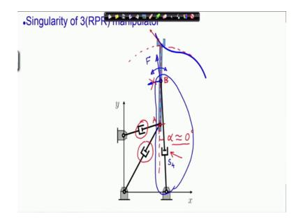
So, let us look at one of these singular configurations, here I have drawn a singular configuration or a configuration very close to singularity, this manipulator is very close to singularity because, the output link and this actuator angle, this angle let me call this alpha is very close to 0. Now why this is singular? Because when alpha is exactly 0 it is a singular configuration and this configuration that I have drawn is very close to singularity.
