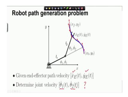
So, the way we will proceed is that given the path we can differentiate at every point and determine the velocity of the end-effector at a specific point on the path. So, here we can differentiate and find out the velocity as a function of time and using the velocity analysis we are going to determine the joint velocity which comprises in this case is theta 1 dot and theta 2 dot.
