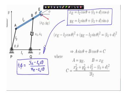
So, these are the relations; you can find out tangent phi. So, tan phi is as equal to y E minus 1 2 sine theta by x E minus 1 2 cosine theta right; from here we can obtain tangent phi and this is what we are going to use.
