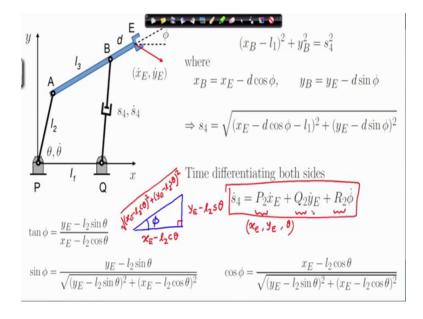
Here, so this is the expression of tan phi. Now once I have tan phi I can also find out cosine phi and sine phi. So, sine phi is this expression, so, how do I find this? Suppose this angle is phi then tan phi is this ratio.
