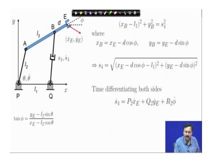
Now, if you differentiate with respect to time both sides of this equation, then you can imagine that you will have derivatives of x E, you will have derivatives of phi and you will have derivatives of y E. And the coefficients corresponding coefficients are P 2 Q 2 and R 2 which can be very easily found by differentiating this.
