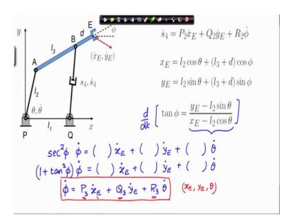
So, here I have re written that expression and I have also rewritten the displacement relation and this expression of tan phi. Now if I differentiate with respect to time I have second square phi into phi dot is equal to the time derivative of the right hand side of this ratio.
