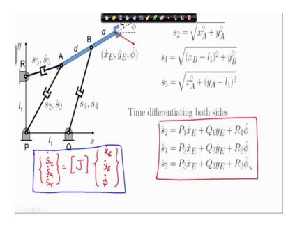
So, if you substitute all these expressions; then finally, you obtain these relations between s 2 dot s 4 dot s 5 dot and x E dot y E dot and phi dot. So, which means I have s 2 dot s 4 dot S 5 dot is equal to a Jacobian matrix times x E dot y E dot and phi dot and
