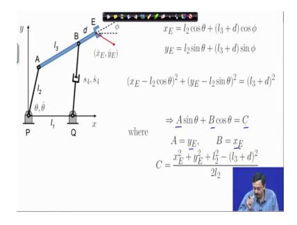
Here I have written out the displacement relations which we have already discussed in a previous lecture. The angle phi; the angle phi is this configuration, this orientation of the end effector; we have also seen in the displacement analysis that given theta and s 4 we can find out x E y E and phi.
