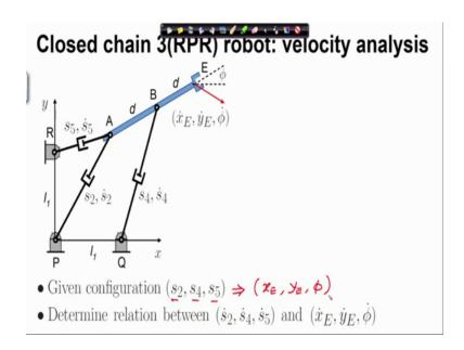
So, let us move forward and discuss the 3 RPR planar closed chain robot manipulator. Here we need to recall that we had already discussed the displacement analysis the configurations s 2 s 4 s 5. So, given s 2 s 4 s 5; the configuration of the manipulator is specified and we have we had found x E, y E and phi.
