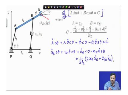
So, given x E and y E we can solve for theta. Now what we are going to do with this relation is that we are going to differentiate this with respect to time. So, this relation we are going to differentiate with respect to time. Then what we have is A dot sine theta S theta represents sine theta plus A theta dot cosine theta plus B dot cosine theta minus B theta dot sine theta is equal to C dot.
