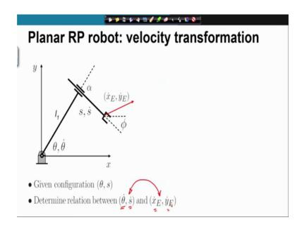
Now, we move onto the RP robot manipulator. Here, our velocity relation was between the joint velocities theta dot and S dot, and x E dot and y E dot.
