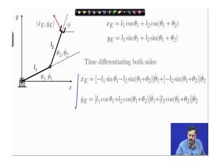
So, we had started off with the forward velocity forward displacement relations differentiated with respect to time to obtain the velocity relations in this form.
