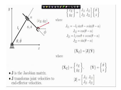
So, in the compact form, we had written out the velocity relations. Here, we have the Jacobian matrix which transforms the joint velocities to end-effector velocities. And to find out the joint velocities corresponding to a desired end-effector velocity, we have this inverse relation.
