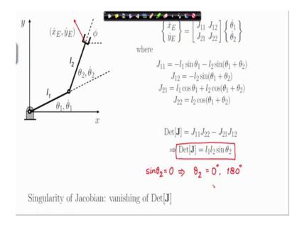
Now, if you take the determinant of this Jacobian for the 2R manipulator, we have this as the determinant. Now, at which point will this determinant vanish, when sine theta 2 is 0, because, 1 1 and 1 2 cannot be 0, so that implies theta 2 is either 0 degree or 180 degree.
