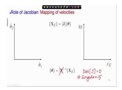
Now, we are going to look at what happens at a singularity. Now, at a singularity as I have mentioned this does not exist. So, Jacobian inverse does not exist, that means, the determinant of the Jacobian has actually vanished. So, this implies singularity, singularity of the Jacobian. And we also say that is the singularity of the configuration of the manipulator. So, we do not have the inverse relation.
