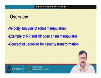
So, we are going to look at the velocity analysis problem for robotic manipulators. I am going to look at two examples RR and RP open chain manipulators and I will also introduce the concept of the Jacobian for velocity transformation.
