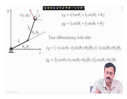
Now, starting with these forward kinematic relations if you differentiate with respect to time then you relate the rates at which xE is changing with the rates at which theta 1 and theta 2 will change similarly for yE.
