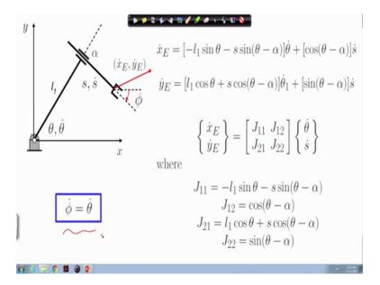
Here I have differentiated these expressions with this involves the joint angle rate and the expansion rate of the prismatic actuator and this can again be assembled in terms of this Jacobian matrix whose elements can be read out from the above expressions. Here the orientation rate of the end effector is just the joint rate of the manipulator this is because the angle alpha is a constant.
