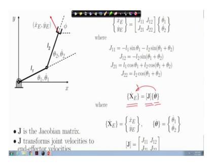
Now, this matrix J that relates the end effector velocity vector with the vector of the joint velocities is known as the Jacobian; the Jacobian matrix. Now Jacobian matrix therefore, transforms the joint velocities to the end effector velocity.
