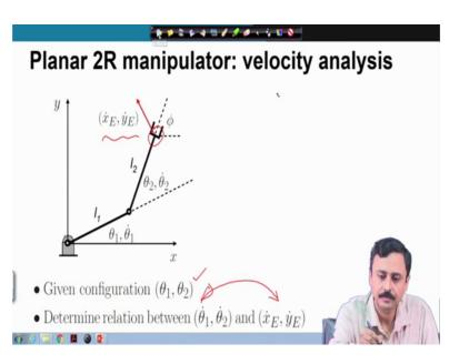
So, this is a 2 R manipulator we are given the configuration. So, configuration needs to be given this comes from the displacement analysis we have to find out a relation between the joint rates the joint angular rates and the end effector velocity vector. So, the velocity of the point, this point of the end effector so, which is specified by this vector x E dot y E dot.
