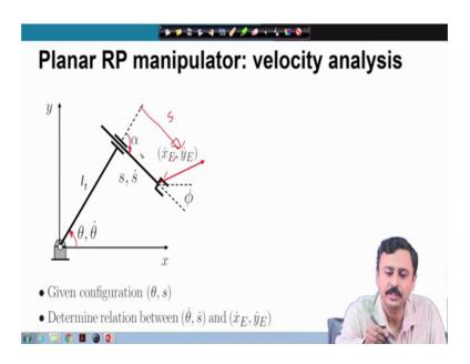
Next we are going to look at the RP manipulator in this manipulator we have this angle as our variable and the through of this prismatic actuator as the other variable. The angle alpha is fixed note that angle alpha is being measured in the clockwise sense therefore it is to be treated as a negative angle.
