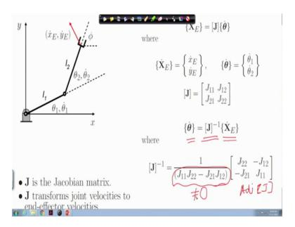
Now, given so, so that is the forward problem now given the end effector velocities how to find out the joint velocities? This is just by inverting the Jacobian matrix, but something has to be borne in mind in order to invert the Jacobian matrix which relates.
