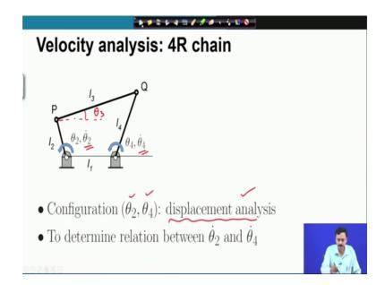
So, as I mentioned that the displacement analysis is completed this is completed. So, which means I know theta 2, I know theta 4 and I also know theta 3, this is displacement analysis. Finding out all these angles given one of them; so, if theta 2 is given I can find out theta 4 and theta 3 or if the output angle theta 4 is given I can find out theta 2 and theta 3. The problem now is to determine the relation between theta 2 dot and theta 4 dot. So, that is the velocity analysis problem.
