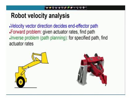
So, in the case of robots we have looked at this we have defined the problem of velocity analysis and its complexity. So, this is intimately related with the path planning or path generation problem in case of robots which we are going to look at in subsequent lectures.
