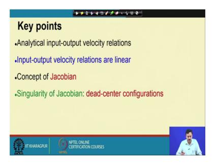
So, what we have observed is that the input output velocity relations are linear. We have used the concept of Jacobian, we have looked at the singularity singularities of the Jacobian which correspond to the dead center configurations. We have done all this for the 4R chain.
