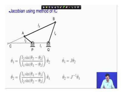
So, let us compare the Jacobian obtained using the method of instantaneous center of rotation. So, you remember that theta 4 was theta 4 dot was related to theta 2 dot using the angles theta 2 and theta 3 and the inverse relation is also given here.
