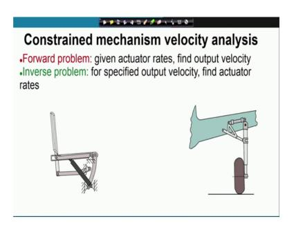
So, we are aware of the velocity analysis problem which is to find out the input output velocity relations; that means, between the actuators and the outputs which is the end effector or the output link. We have these two problems; forward and inverse problems given the actuator rates, finding out the output velocity is the forward problem and given
