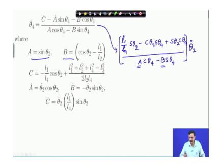
So, if you just substitute in here, so, C dot is 1 1 by 1 4 sine theta 2; I will take out theta 2 dot and A dot is cosine theta 2 sine theta 4 and this is plus sine theta cosine theta 4 this whole thing getting multiplied by theta 2 dot.
