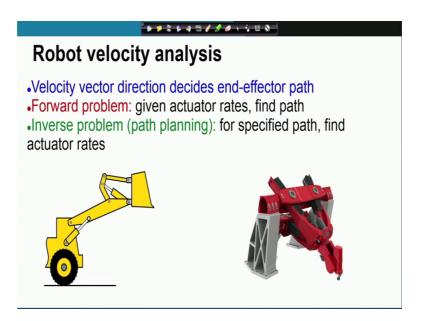
In the case of robots, we have seeing that velocity analysis problem is little more complicated, where we need to specify the velocity along a path, because the velocity vector will always be tangent to the path and corresponding to that velocity vector. We can find out the actuator rates through the velocity analysis by solving the velocity analysis problem.
