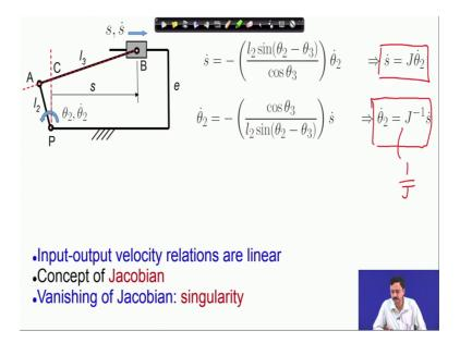
So, I will write this in a compact form as I have done here. So, s dot is the Jacobean times theta 2 dot and by inverting the Jacobean can write theta 2 dot is Jacobean inverse,
