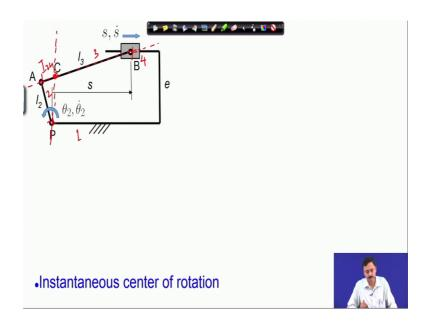
So, for this as I have mentioned, we are going to use the geometric concept of instantaneous center of rotation. So, the instantaneous center rotation that I will use for this analysis is I 2 4. So, this lies on this line passing through I 2 3 that mean mark out this is 1, this is 2, this is 3 and the slider is link 4. I want to find out I 2 4.
