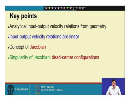
So, let us recapitulate the key points. We have found the analytical input output velocity relation from geometry. Now here I must mention again that we have use the concept of instantaneous center of rotation of the mechanism and then from geometric relations we have try to find out certain lengths.
