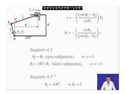
So, I have written out these velocity relations again. So, singularity the Jacobian occurs when theta 2 equals equal to theta theta 3. The singularity is an open configuration 1 where S dot 0 or you can also have singularity when theta 2 is 180 degree plus theta 3, in which we have the folded configuration, in which also S dot is 0.
