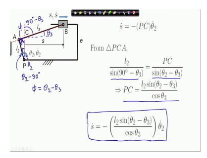
Now, we have to find out P C. To do that, we look at triangle PCA. So, you can that easily find out PCA and use the sin rule. You can see that 1 2 divided by this angle. Now what is this angle? Remember that this is theta 3. So, that angle that link 3 makes with the x axis or the horizontal axis is theta 3. So therefore, this angle must be 90 degree minus theta 3.
