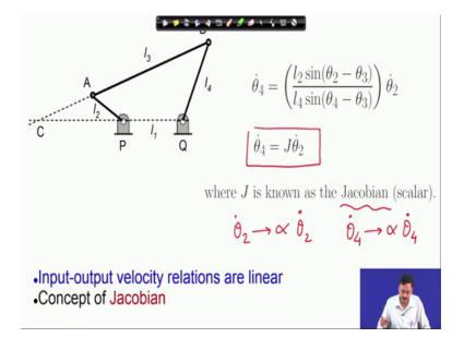
Now, this relation between theta 4 dot and theta 2 dot I will write in a compact form as theta 4 dot is equal to J times theta 2 dot this J is known as the Jacobean here this is a scalar quantity. That means, it is a number given theta 2 or having known theta 2 theta 3 theta 4 I can exactly calculate this number which is J this is called the Jacobean.
