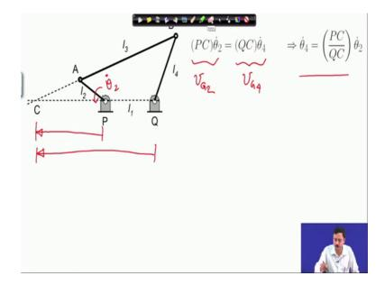
So, I have located for you I 2 4 which is the point C. Now you can very easily from geometry write this expression that PC which is this distance PC times theta 2 dot. What is this? This is nothing but velocity of G 2 PC times theta 2 dot. So, this is theta 2 dot must be equal to QC times theta 4 dot this is the condition. So, this is V G 4; now this is the condition that first we satisfied at I 2 4.
