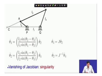
So, there are very special configurations at which such conditions are met. So, vanishing of the Jacobean is called the singularity of the kinematic chain or the mechanism. So, we will spend a minute some minutes discussing this vanishing, because this is very important. And I will relate this to one of the previous concepts that we have used which is the dead center configuration.
