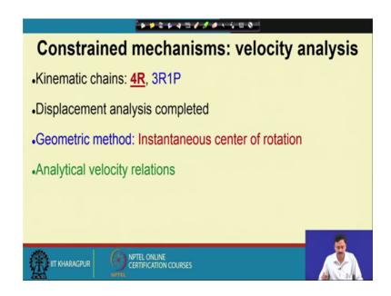
So, in this lecture we are going to look at the 4R kinematic chain. We will assume that the displacement analysis is completed. In other words I know the configuration of the mechanism this is a very important point. So, before I embark upon the velocity analysis problem I must have the displacement analysis problem completely solved. In other words I should be able to find out the configuration of the mechanism or I should know the configuration of the mechanism.
