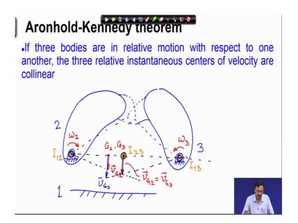
So, we are going to start by just reviewing the Arnold Kennedy theorem which states that if three bodies are in relative motion with respect to one another the three relative instantaneous centers of velocity are collinear. So, just to explain this once again let me consider three bodies. So, two and the third one I will define like this that, suppose this is the instantaneous center of rotation of let me call it body 2.
