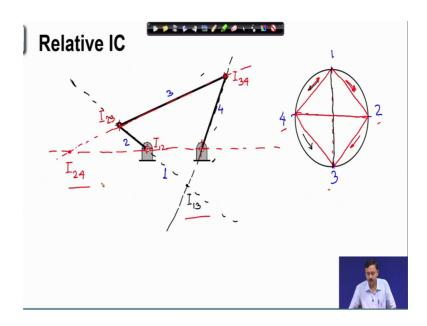
Now, let us apply these concepts in mechanisms. So, we will try to locate the relative IC's for this mechanism, let me number the links first so ground is 1, this is 2 3 and 4. Now to locate all the relative IC's we have what is known as the circle diagram. So, I will mark the number of links so 1, 2, 3, 4; so 1, 2, 3, 4. So, we have 4 links. So, I will mark 4 points on the circle, I will join the 2 2 points if I exactly know the relative IC between those two bodies.
