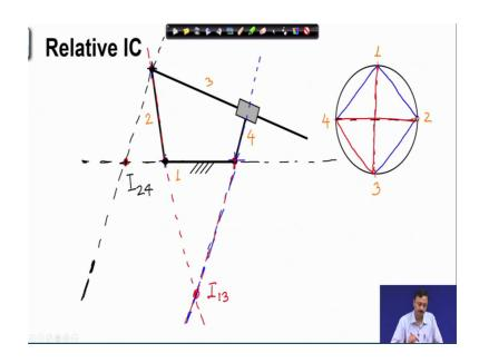
Let us move to the next mechanism. So, let me number 1, 2, 3 and 4. So, there are 4 links. So, four points on our circle diagram I know the IC between 1 and 2. So, I 1 2 is known I 2 3 is also known, I 1 4 is also known. Now I 3 4 must lie on this line which is perpendicular to the sliding direction.
