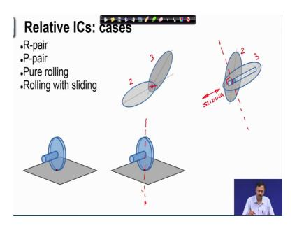
Which we have seen before so this is the relative IC between bodies 2 and 3, the revolute pair for the R pair the revolute pair itself is the relative IC between 23 in the case of a prismatic pair the relative IC between the bodies 2 and 3 lie on this line which is perpendicular to the direction of sliding.
