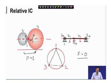
Here is the final example, here I have a chain with three links now I. So, this is two this is three ground is one I know I 1 2 I know I 1 3 and in both cases I also know I 2 3. So, this is in pure rolling. So, this is the IC of two related to 3. So, this is in the case here it is I 1 2 this is I 1 3 and this is I 2 3, but then you know this mechanism in which you have two friction disk they can continuously roll they this has one degree of freedom.
