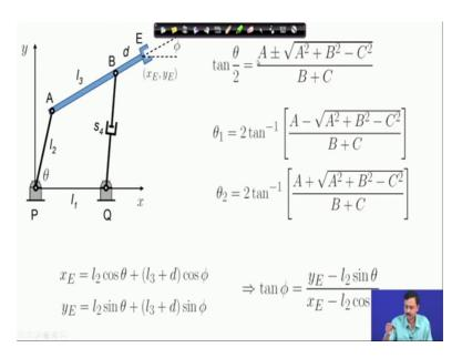
So, formally so this is the expression for tan phi. So, from here I can solve for phi, again using the a tan 2 function because I need to get the quadrant right.
