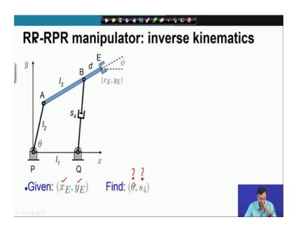
Now let us move on with the. So, this is the RR-RPR manipulator and we are going to study the inverse kinematics of this chain now. Here we are given the coordinates of the end effector and we are to find out the inputs the actuator inputs, which are given by theta and s 4.
