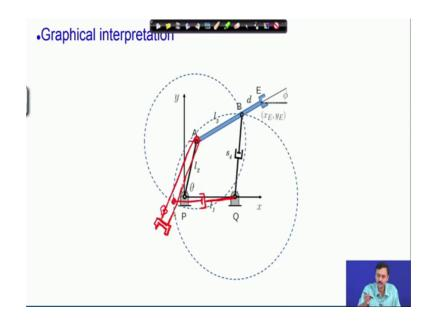
Let us understand the solution graphically, remember that we are given theta and s 4. So, therefore so theta and s 4 are given. Now if you see when theta is given then this point A gets fixed, what is not fixed is phi because this hinge B on the end effector link can rotate on this circle, while the hinge B on the actuator arm on this on this other leg can rotate on this circle.
