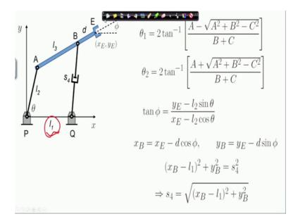
So, this is what I have written out. So, s 4 is square root of x B minus 1 1. So, you have 1 one here the length P Q. So, x B minus 1 1 whole square does y B square because y Q is 0 the y coordinate of point Q is 0.
