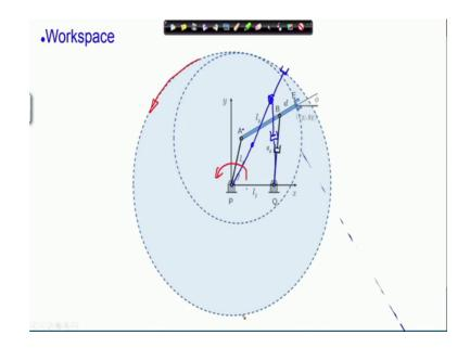
This is the workspace of the manipulator. So, if you completely extend, if you completely extend this link and then move it in the circle, you generate the outer circle which defines the workspace of this manipulator. Of course, with joint limits or actuator limits this workspace is going to get more complicated and will be reduced which you can find out based on geometry.
