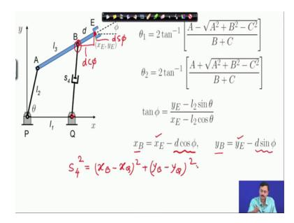
So, I have corrected these expressions now. So, we know theta 1, theta 2 in terms of x E y E then I calculate phi, once I have phi I can define the coordinates of point B. So, coordinates of point B is nothing, but coordinates of point E which is the end effector point which is given to me, which is known minus this d cosine phi which is the projection of B E this is a projection of B E along the x axis.
