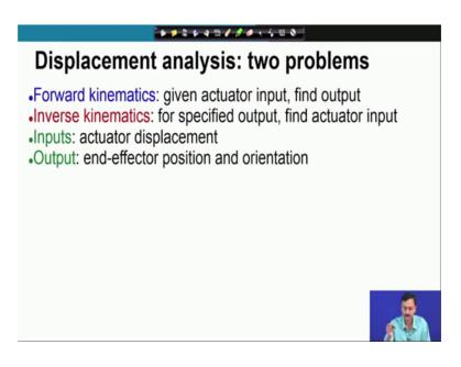
Now, we have two kinds of problems as you know the forward kinematics problem in which the actuator inputs are given, we have to find out the output, output is the end effector position or position and orientation depending on degree of freedom of the chain.
