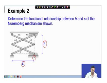
So, this example asks us to determine the functional relationship between h, which is the height of the platform, and s which captures the displacement of the slider pin be A. Essentially the location of A is captured by s and correspondingly h is the height of the platform; so, to determine a functional relationship between h and s.
