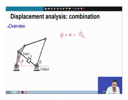
Therefore, we can solve this to find out phi. Once, I know phi, then I identify the angle phi plus alpha as let us say theta 2, it is only phi.
