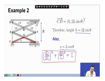
Now, we have two stages in this mechanism this and this, both are L sin theta. Therefore, the total height is 2L sin theta, and we have s equal to L cosine theta. We have two relations h as 2L sin theta, and s as L cosine theta. If we eliminate theta between the two, which is done this way h by 2L is sin theta, so sin the square theta plus s over L is cosine
