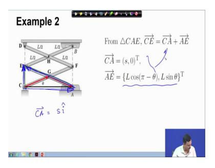
From triangle CAE, this is this triangle CE this vector must be equal to the vector CA plus the vector AE. Now, CA the vector CA is nothing but s i cap in the coordinate system, we have chosen. And AE this vector can be represented in this form, therefore substituting these two here.
