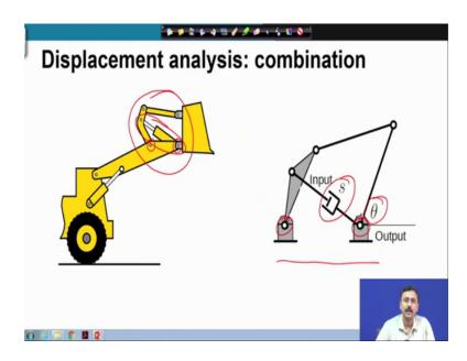
Let us look at another example. This I will discuss given idea of how to solve the displacement analysis problem for more complicated mechanisms. Here I have considered this part of the mechanism, which is represented here. I have made these two hinges as the ground hinge of this mechanism, there are two ground hinges.
