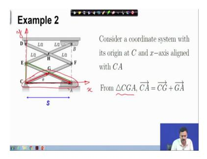
We consider a coordinate system; this is x y coordinate system. Now, from this triangle CGA, so this triangle; now, C A you can easily read out, C A is equal to the vector C G plus vector G A.
