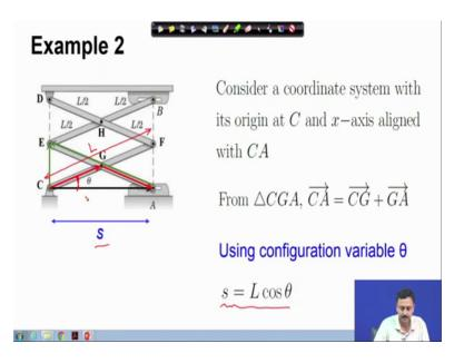
We use this variable theta this angle, therefore this s this displacement s is equal to L cosine theta, where L is this length of this link. So, s equal to L cosine theta.
