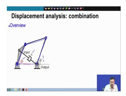
If this is phi, then we can look at this chain this 4 r chain. Look at this 4 r chain, where phi is known. We have to find out theta, which is the problem which we have already solved. Therefore, using two steps you can find out theta given s. So, first we find out phi, and from there we find out theta.
