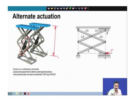
There can be alternate actuation mechanism as shown here, rather than applying force here. This is one possibility, you apply a force here and shift pin A. There are other possibilities, you can have prismatic actuators arranged like this here also from geometry, you can determine the relation between the actuator throw and the height of the platform.
