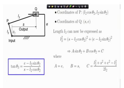
So, as we have discussed before, we consider coordinate system theta 2 is the angle made by the link 1 2 with the x axis. Therefore, you can easily read the coordinates of point P which is this one as 1 2 cosine theta 2 and 1 2 sin theta 2. So, P x is 1 2 cosine theta 2 and P y is 1 2 sine theta 2. The coordinates of Q which is the slider; the x coordinate is e, the x coordinate is s and the y coordinate is e.
