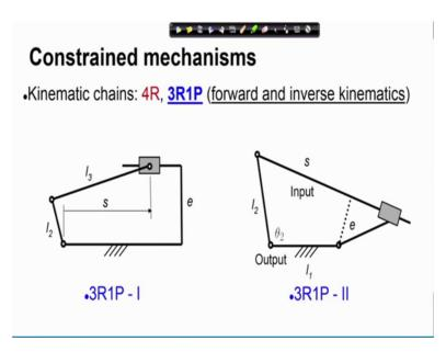
So, in this Constrained Mechanisms, today we are going to look at 3R1P chains. So, there are two 3R1P chains as shown on the left I have 3R1P chain 1 and on the right, I have 3R1P chain 2; they are essentially inversions. But there are Displacement Analysis, they differ in certain ways.
