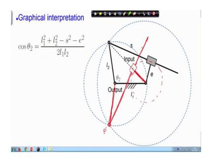
Let us look at these two solutions graphically. Remember that s is specified. If s is specified, then this P Q length is fixed. This is P Q. This length is fixed, but what is not fixed are this angle theta 2 and also this angle. Therefore, when I change theta 2, the point P will move on this circle; when I change theta 2, the point P will move on this circle; when I change theta 2, the point P will move on this circle.
