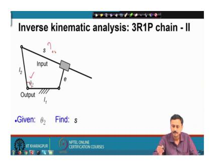
Now, we go over to the Inverse kinematic analysis of 3R1P chain type 2. Here, we are given theta 2. So, this theta 2 is given we have to find out s. Let us look at this triangle P Q R.
