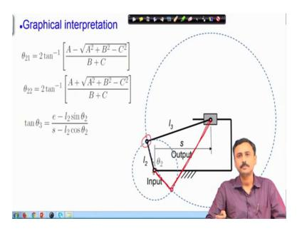
Now, we look at the interpretation of the solutions there are two solutions as we have mentioned. In this case, I am given s. Therefore, this point is fixed, the slider position is fixed. We can now think of assembling the mechanism by looking at the location of this hinge P. This P is a point on link 1 3 will move on this circle larger circle; whereas, P as a point on the link 1 2 will move on this smaller circle.
