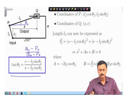
I can obtain this quadratic equation in s which can be solved because I know these coefficients A and B in terms of theta 2 and the other link lines because A and B are known to me I can solve for s.
