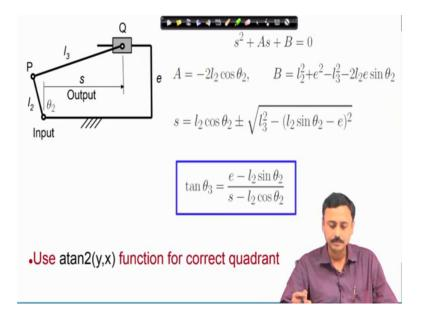
Finally, I have put together all these equations which can be solved[noise] now easily to find out s, and finally theta 3. Now when you solve for theta 3, remember to use the atan2 function which gives the correct quadrant of theta 3.
