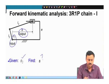
Let us start with the Forward kinematics analysis of this 3R1P chain type 1. So, in forward kinematics, as I have mentioned before that we are given the input we have to find out the position of the output link? Here, the input as shown is theta 2 and the output is s input is theta 2 and output is s: s is the displacement of the slider from a certain coordinate in a certain expressed a certain coordinate system.
