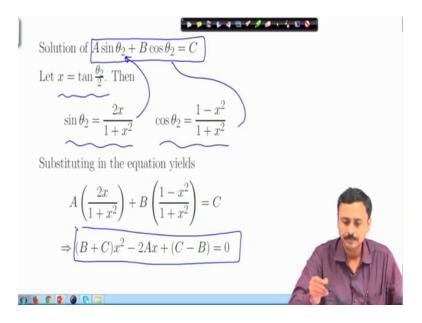
So, we now have to solve this equation for theta 2. We make this substitution x is equal to tan theta 2 by 2 and write sin theta 2 and cosine theta 2 in terms of x and substitute these expressions in our equation to be solved. And finally, obtain this quadratic equation now in terms of x.
