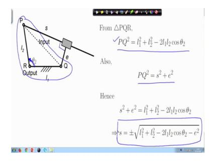
And the cosine rule, I can very easily write P Q square as 1 1 square plus 1 2 square minus 2 1 1 1 2 cosine theta 2 theta 2. Remember that theta 2 is specified. Therefore, I can find out P Q. I know P Q. Now P Q square is s square plus C square. This being 90 degree. Therefore, I have 2 solutions of s from here given by plus or minus. Now let us look at the interpretation of these 2 solutions.
