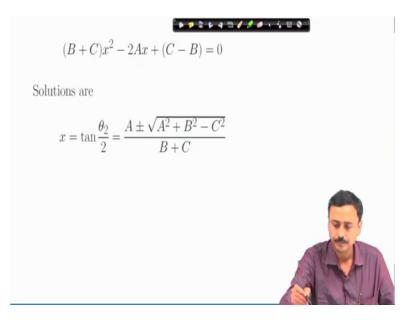
We know the solution of a quadratic equation. The solutions there are 2 solutions like this and the solution of x; x is essentially a tan theta 2 by 2. So, we have 2 solutions of theta 2.
