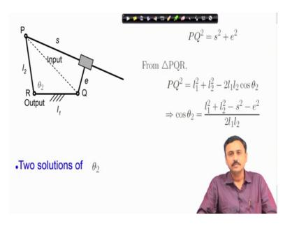
First, we will discuss the Forward kinematics problem. In this problem, we are given the input. Input is usually as you have seen input is usually the hydraulic actuator. Therefore, this is given s is given which is the input and we have to find out this angle theta 2 which is the output.
