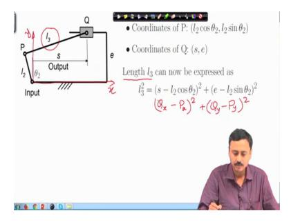
Given the coordinates of P and Q, the length 1 3 which is this link essentially the length of PQ: so 1 3 square can be written as this is Q x minus P x whole square plus Q y minus P y whole square and that is 1 3 square. Now, if you open this up considering that we are given theta 2 and we have to find out s; I can obtain this quadratic equation in s.
