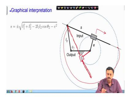
So, I have written out the solution of s plus plus or minus this quantity. Now, plus is interpreted as a displacement in this direction. This is positive s and of course, this is negative s.
