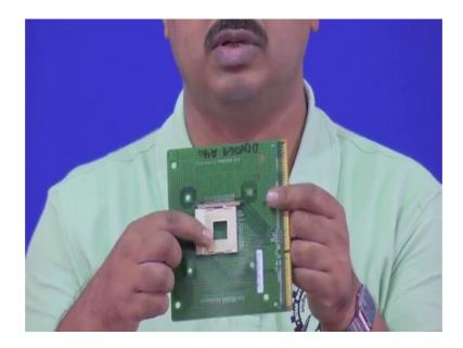
This is the package or the substrate on which the pins are attached right and then this goes inside a socket like this, as we had seen the last time ok. The pins will perfectly fit in these sockets which has corresponding holes.
