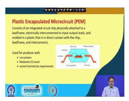
So, that brings us to the next slide, which is plastic encapsulated micro circuit or PEM ok, this is nothing but plastic chip carrier. Again I am going to show sometimes these different acronyms, because these are widely used in the electronics industry. But, what it essentially means is this configuration, which is plastic chip carrier. But, the only thing
