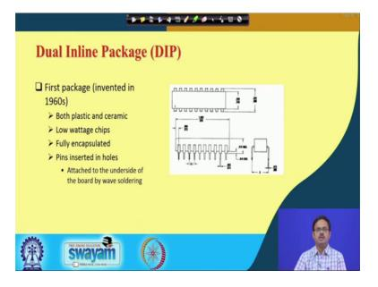
So, after plastic and ceramic packages and chip carriers. Let us move on to something called a dual inline package, which is something we saw ok, it can be plastic, it can be ceramic. But, what is important is this was the first package that was invented in the 1960s.
