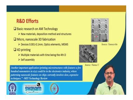
And, lots of R and D efforts are going on new materials, deposition method structures. Micro nano scale of 3D D in micro nano scale 3D fabrication devices of the order of you know 0.1 millimetre to 0.001 millimetre some 1 micron possible. Optical elements, MEMS: Micro Electro Mechanical Systems you see these in Vienna University what they have made these are in microns ok, nano scribe another one.
