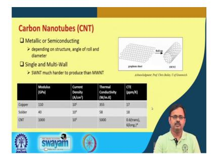
So, lead free solder has been a big there has been a big push towards first of all coming up with new materials and characterizing them under different applications alright. The second special topic we wanted to discuss is carbon nanotubes. What is carbon nanotubes? Carbon nanotubes is if you take what is called a graphene sheet which is a 2D carbon a allotrope; primarily from graphite what is graphene and then if you can roll it up in this manner what you get is a carbon nanotube ok.
