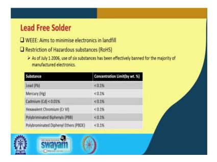
So, lead free solder, what does this mean? So, see all this file whatever solder traditionally we have used since we started using electronics and making electronic components, the solder has primarily been lead tin solder ok; lead and tin where the primary components. But however, what happened is RoHS which is Restriction of
