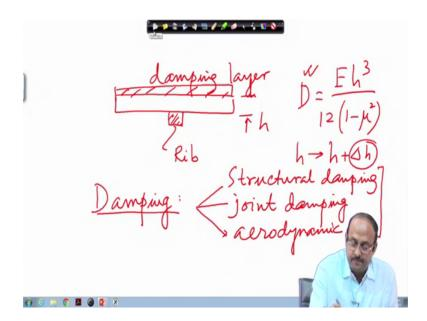
Now if you consider the plate which has certain thickness and then so this is the h D will be equal to E h cube divided by 12 1 minus mu square. Now, if you increase the value of the h definitely the value of D increases and so increases omega n. Now, PCBs cannot the thickness of the PCBs cannot be increased to a large extent, but what we can do we can attach rib over there.
