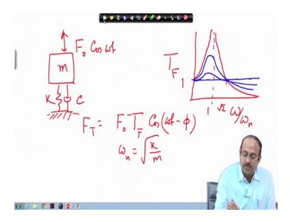
So, if you have a vibrating system which may have certain damper. So, m K C if this is actually excited by certain force F naught cosine omega t then there is force transmitted to the so this is our system and this is our structure and this is the system which should not be excited by that much of force.
