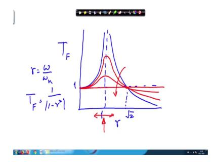
Now, let us see how the transmissibility behaves. So, if I plot omega by omega n r equal to omega by omega n and here it is transmissibility T F. So, transmissibility is 1 by 1
