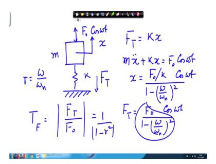
So, let us first consider the force transmissibility. We have a vibrating system and here there is the spring and the mass. And, this is supposed excited by harmonic force F naught cosine omega t. Now, if you write down the force transmitted; that means, what
