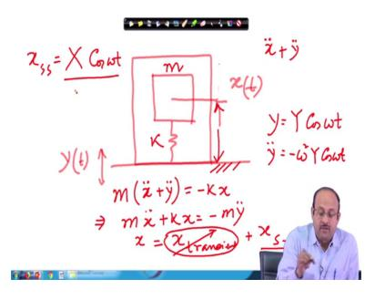
Now, when we have a steady state steady state motion; that means, let us consider now the situation where we have again similar box and this is actually the box. And, this is connected to a table and this table is actually getting vibrated with a certain motion y t, then what is going to happen. So, here if I consider x t and this x t suppose this x t I measured not from here, but let us say this is our x t that is the measure from the base.
