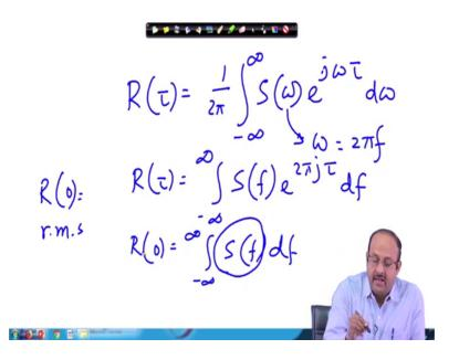
This is equal to 1 by 2 pi and S omega e to the power j omega tau d omega minus infinity to infinity. Now, sometimes instead of omega which is the circular frequency we write down in terms of the frequency hertz. Then in that situation R tau will be equal to minus infinity to infinity S is a function of f and e to the power 2 pi j j tau and d f.
