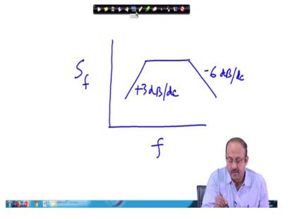
Now, in many situations when we have rms value that is in many cases the y is specified in terms of its rms value. If we have f then the rms value of this thing; that means, we consider S f. And in many cases the function is something like this for example, when we in a in a standard testing protocol will have S f function is kind of this is increment is 3 dB maybe this is minus 6 dB or so.
