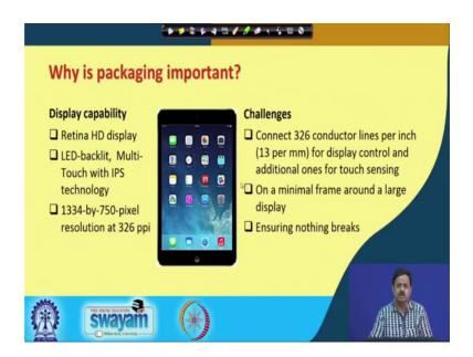
Second, this is the processor. So, to make the to make the maximum use of the processor capability ok. Display capability, yes we have display technologies that has really gone in leaps and bounds over the last few years we have retina high I mean HD display, we have led backlit display with multi touch sensing with IPs technology. We have really high definition display these days 1334 by 750 pixels now I think it is even more.
