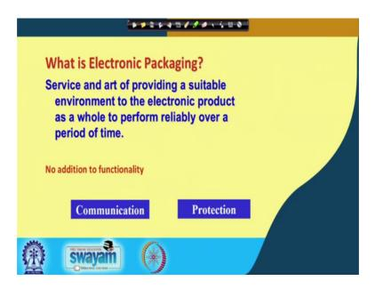
So, what is electronic packaging? If you refer to the slide that I showed in the last class, is the service and art of providing a suitable environment to the electronic product as a whole to perform reliably over a period of time ok.
