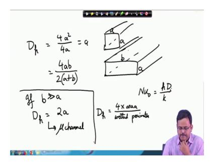
So, let us go over here what will be D h for a square it is 4 a squared 4 times area. So, the flow is this is the cross section of the pipe right instead of a circle, 4 a squared over 4 a equals 2 a. What happens if it is a rectangle? Think about it this is very similar to flow between 2 fins through a channel then what happens 4 a b divided by 2 into a plus b ok.
