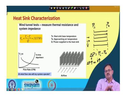
These are my adjacent fins and I am having an airflow at V dot. So, if I take a cross section here, I will measure a pressure P i which is an inlet pressure. And if I do the same over here I will measure a pressure P naught and delta P which is a pressure drop is going to be P i minus P naught. And this delta P increases as V dot increases ok; now why does this pressure drop happen?
