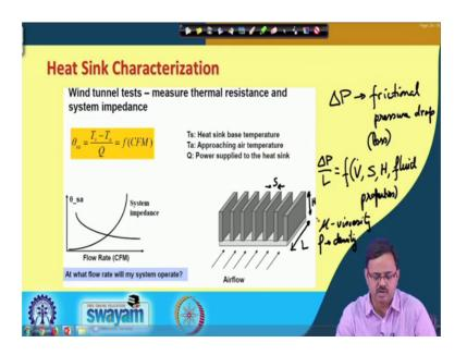
So, that is a little bit into the details, but what I am trying to say is this delta P is typically for flow through a channel; it is a frictional pressure drop. Sometimes it is also called the frictional loss alright; so that is why the delta P go increases you see this increase.
