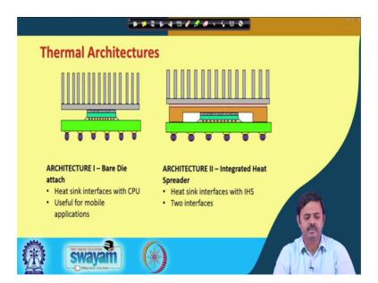
So, now let us look into what is called thermal architecture ok. So, there are two very common thermal architectures for a silicon in the computing world. So, one is called the bare die attached, and one is called the integrated heat spreader ok. So, the first one I am going to talk about is bare die attached. So, here the silicon is this green portion is this one ok, as you can see it is flip chip bonded onto this substrate correct.
