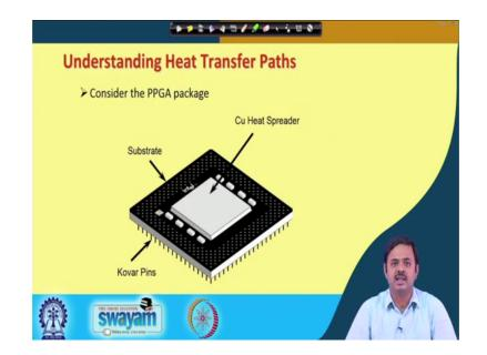
And we will look at one of a simple package, as you can see this is a pin grid array, it is a pin grid array. It is it is a very old Intel package, it is a schematic of that. And what you see is you cannot see the piece of silicon inside, because it is covered with a copper heat spreader, heat spreader is like a plate ok. And we will see a schematic in the cross sectional schematic in the next direction in the next slide ok. So, this is the substrate or
