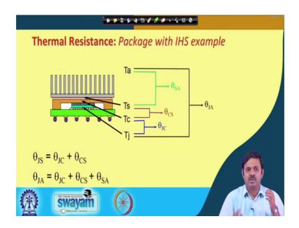
Think about if I want to do measure the temp in the previous slide, if I want to measure the temperature of the sync T s, and T c its impossible ok, where do you put the thermocouples are going to collide with each other ok. So, there are certain disadvantages, but all said and done theta is widely theta JC, theta CA, theta JA, theta JS these are widely used parameters in the electronics packaging industry ok. People use it, engineers practicing engineers use it day-in and day-out.
