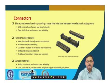
So, next thing is connectors. So, what are connectors we all know what connectors are we use it every day, but it is an electromechanical device providing a separable keep in mind, separable it cannot be a permanent attached I have connected it and that is it, no, I should be able to remove it. So, it is a separable interface between two electronic subsystems. See some, some examples of connectors ok. There are various types that are available.
