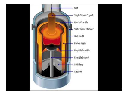
Step 1, preparation of high purity of molten silicon. In Czochralski process high purity of silicon is encouraged to be used as molten to form single crystal silicon. Silicon dioxide can be used to prepare high purity molten silicon then the substance will be heated to it is melting point into a crucible made of quartz. The supersaturated molten solution will become the source of silicon wafer.
