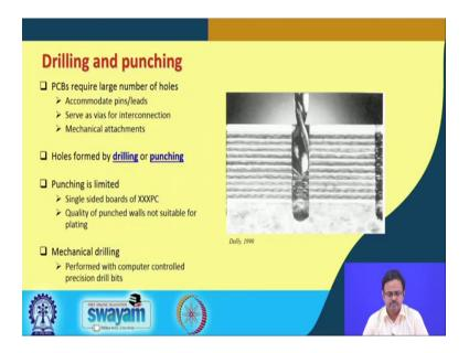
The last thing that I am going to talk about in motherboard or in circuit board is the process of drilling and punching because, PCB's as I said require a large number of holes whether it is for mechanical purpose or whether it is for interconnections or whether it is to accommodate pins. Remember the plated through hole components if it is a two layer motherboard, you can do that right; you can have just through hole going through ok.
