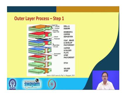
Now what happens? The outer layers, inner layers we have seen what to do with. What about the outer layers? Inner layers already the traces are there, due to up lithography and etching and then they are separated from each other by this prepeg and everything is fine as you can see the inner layers are all fine. This is a 6 layer motherboard, 1, 2, 3, 4, 5, 6; you can see 6 copper traces, but the outer layers still remain.
